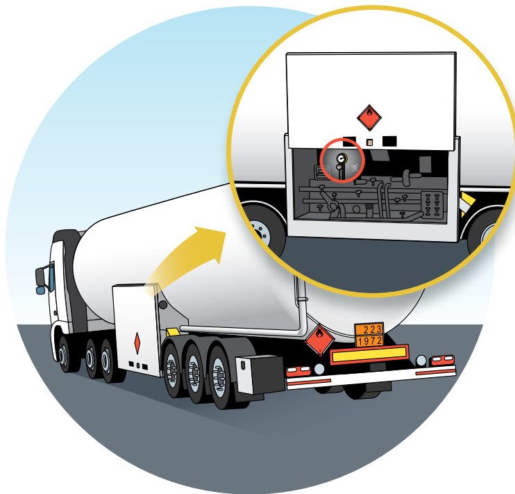
The transport unit's control box contains pressure and level gauges.
